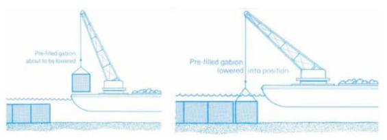
Fig. 39: Underwater Placement of Prefilled Gabions by Crane
