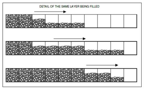
Fig. 33: Filling Pattern of Gabion Boxes
