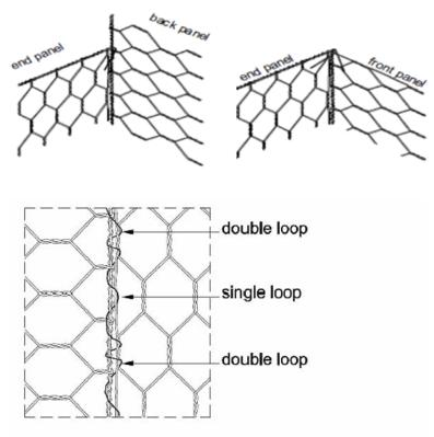
Fig. 31a: Assembling details with Lacing Wire
