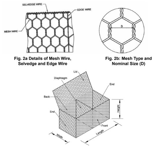
Fig. 2c: Details of Assembled Gabion Box
