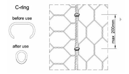
Fig. 31b: Assembling details with C-rings
